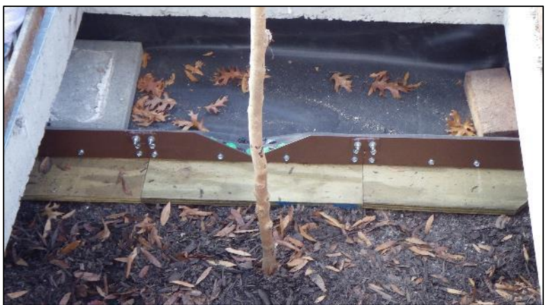
Figure 22. Inflow compound weir for flow measurement
