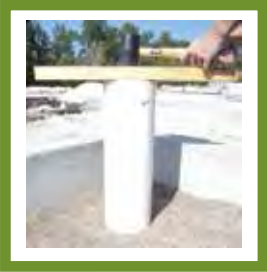
Figure 3: Hammering Pipe Into Media
