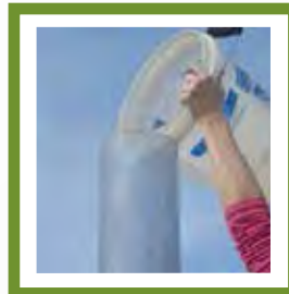
Figure 9: Filling Infiltrator with Water
