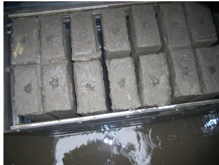
Solid BioMediaGREEN coated with fines
