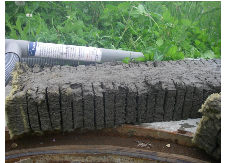
Ribbed BioMediaGREEN coated with fines
