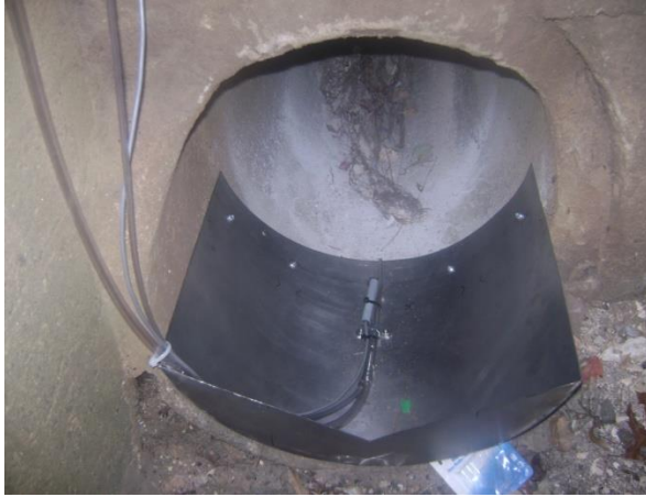
Figure 4: In-Line Monitoring Weir
