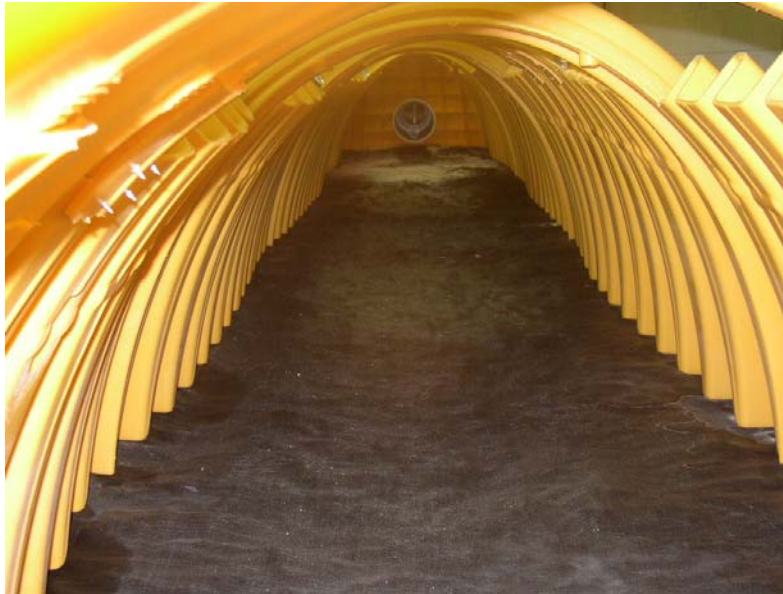
Figure A12.7 - View from fourth chamber looking upstream at the inlet pipe. Notice that all sediment is deposited within first chamber. Hydraulic loading rate = 0.4 \text{ gpm/ft}^2 (7/4/04)
