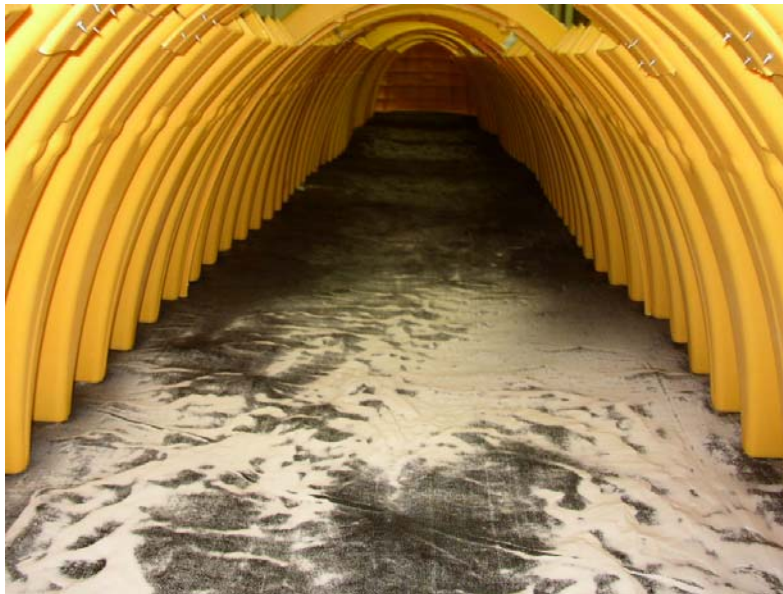
Figure A12.8 – view looking downstream from first chamber. Again, scouring of sediment occurs near inlet, and sediment is deposited mainly in first chamber. Hydraulic loading rate = 0.4 \text{ gpm/ft}^2 (7/4/04)
