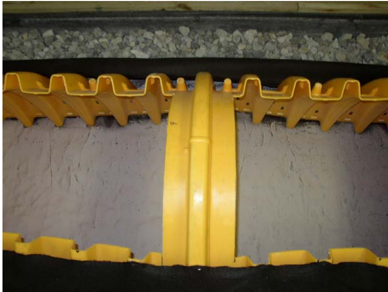
Figure A12.6 – Overhead view of middle chambers with largest volume of sediment. At this high flow, sediment distribution was particularly uniform. . Hydraulic loading rate = 4.84 \text{ gpm/ft}^2 (6/19/04)
