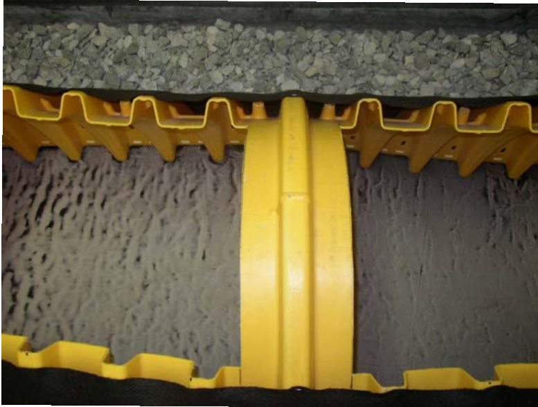
Figure A12.3 – Overhead view of middle chamber containing the largest amount of sediment. Hydraulic loading rate = 1.61 gpm/ft 2 (6/29/04)
