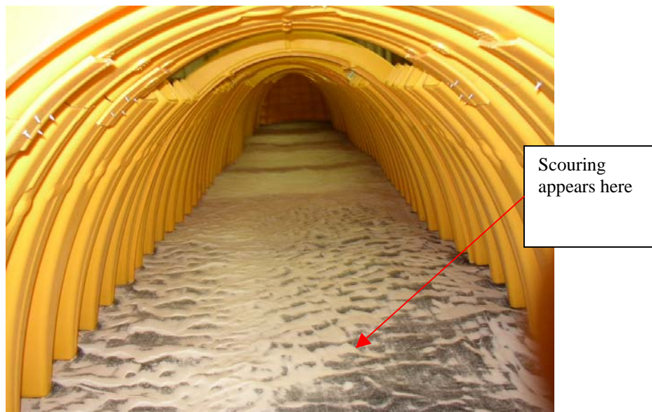
Figure A12.5- view looking downstream from first chamber. Again, scouring of sediment occurs near inlet, however, not to the degree of the lower flows. Hydraulic loading rate = 4.84 \text{ gpm/ft}^2 (6/19/04)
