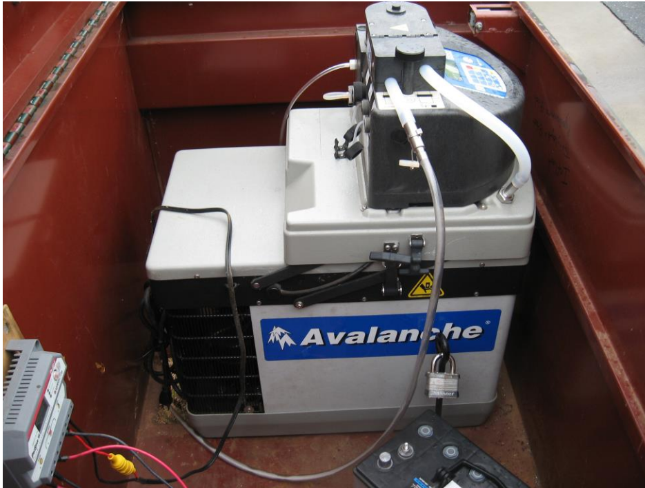
Fig 3.1 ISCO Avalanche Model 6712 sampler
