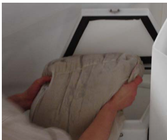
Figure A-5: View showing media bag with Filter Sand being installed in the Filter Module
