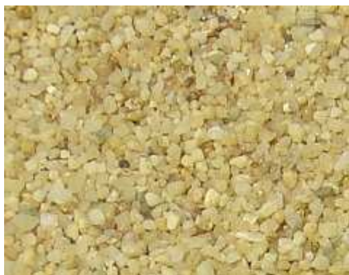
Figure A-6: A close-up view of the Filter Sand
