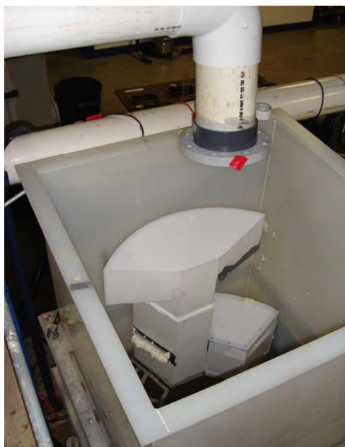
Figure A-3: View Showing a One-Filter Module Set-Up
