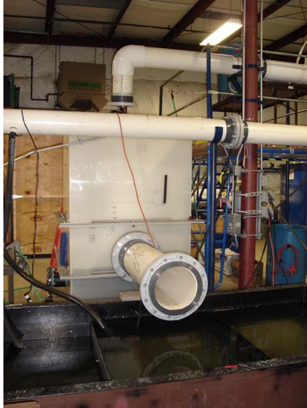
View Showing Up-Flo™ Filter Overhead Inlet Pipe, Outlet Pipe and Collection Basin
