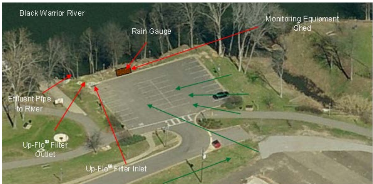
Figure 8 Location of Monitoring Equipment at Bama Belle Site
