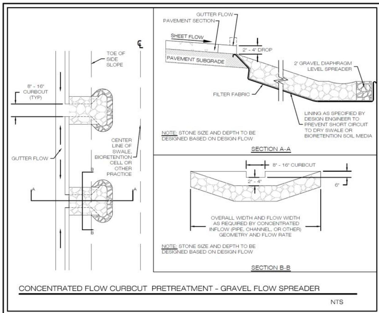
**Figure 9.9: Pre-Treatment – Gravel Flow Spreader for Concentrated Flow**
