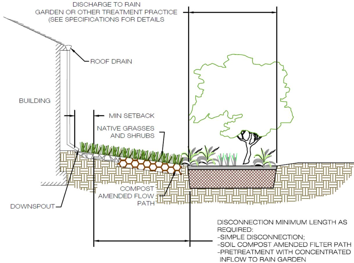
**Figure 9.3A. Residential Rooftop Disconnection – Section View:**
