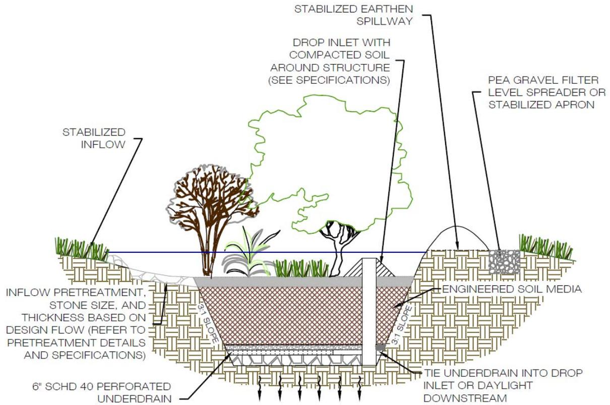
**Figure 9-B.4. Typical Bioretention Basin – Inflow & Outflow - Section**
