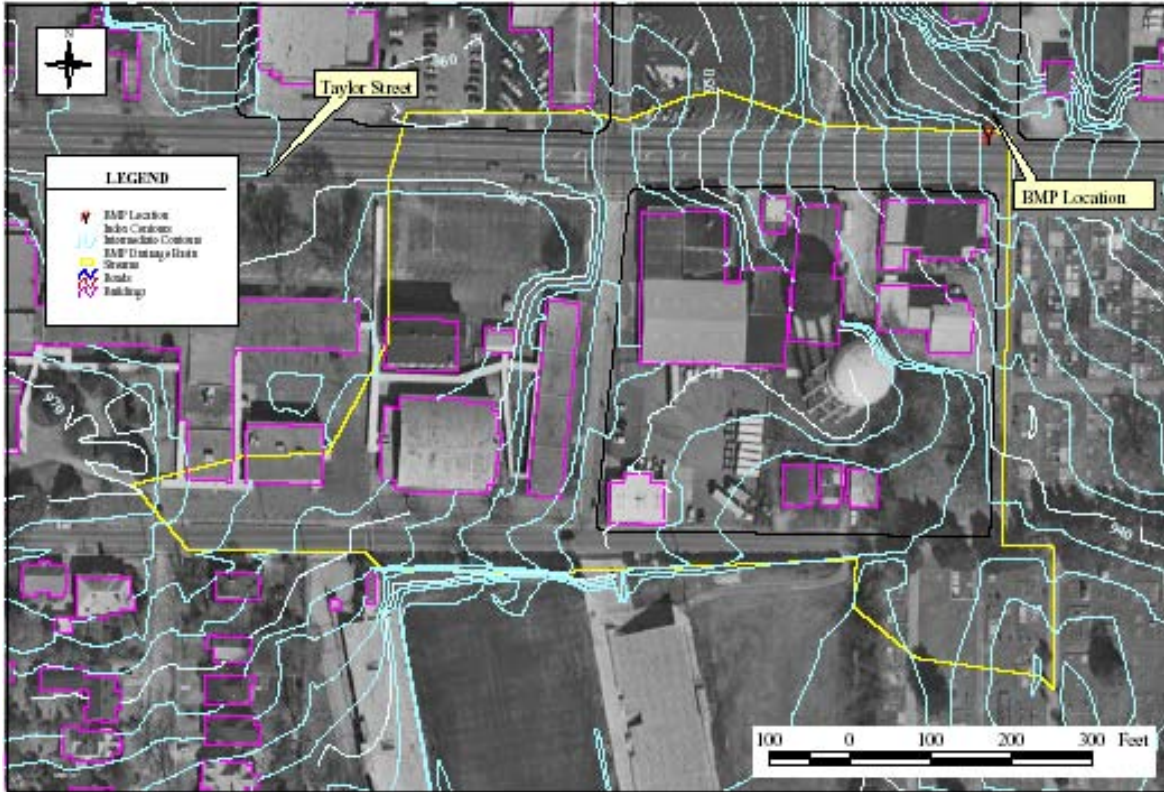
Figure 3-2. Drainage basin map for the BaySaver installation.
