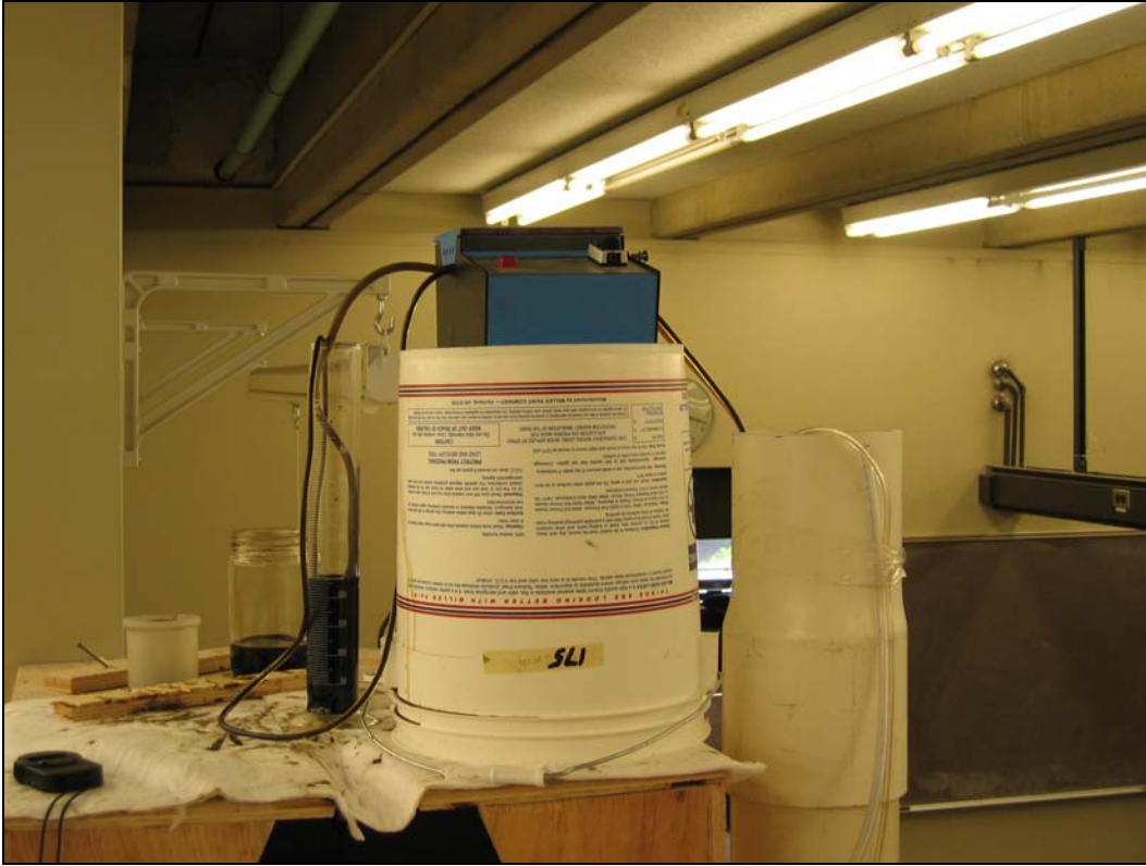
Figure 15. Peristaltic pump and oil inlet
