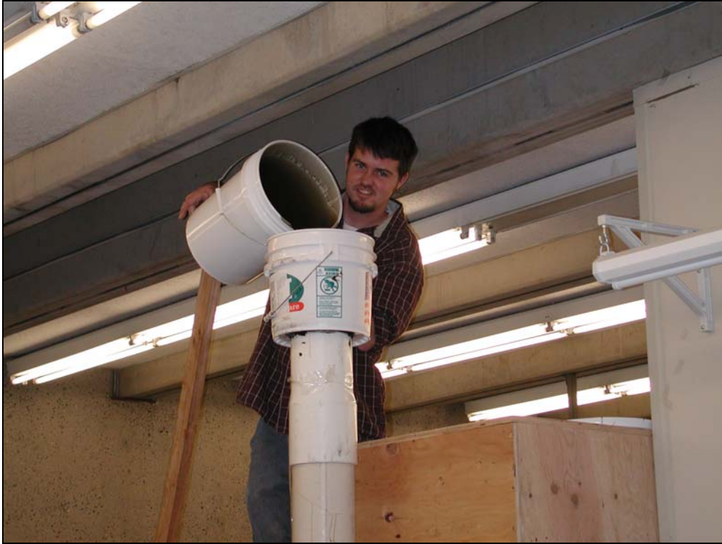
Figure 21. Adding oil in for the dump test
