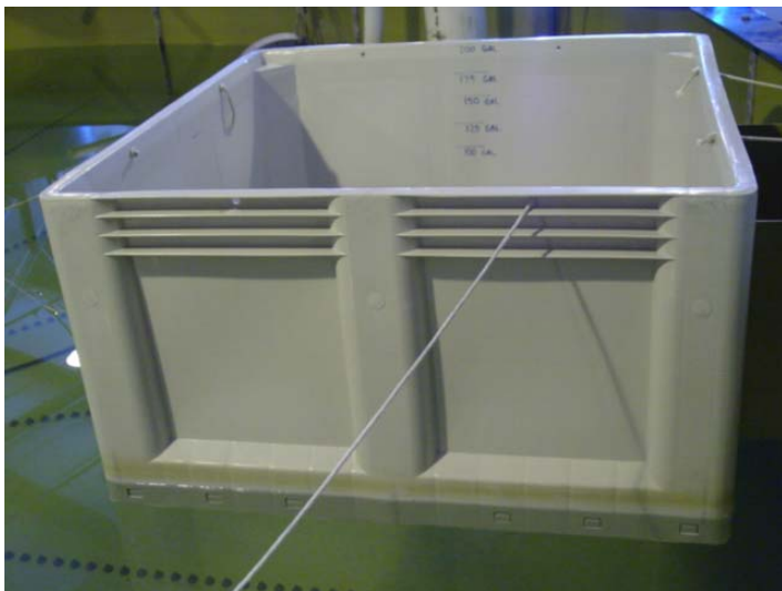
Volumetric Time-To-Fill Tank
