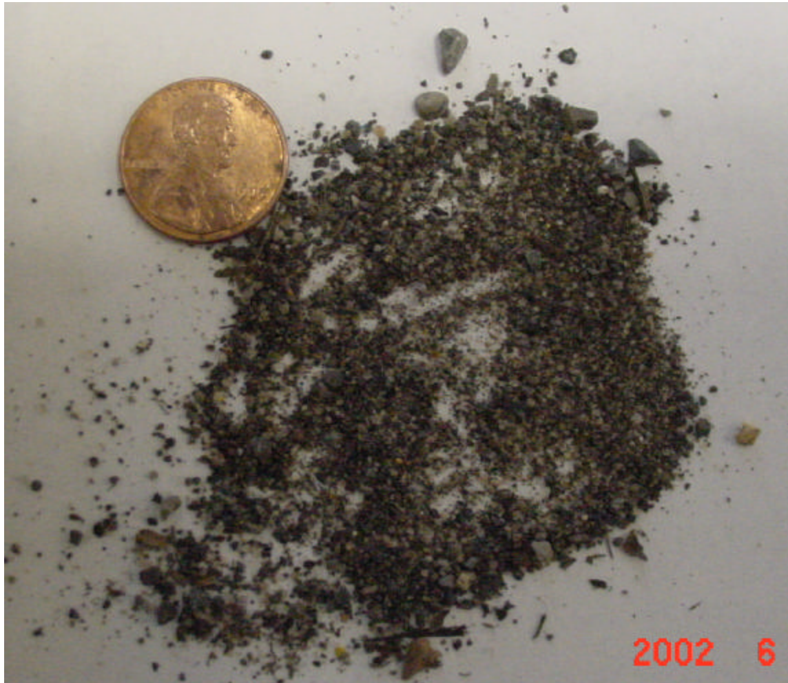
Influent Stormwater Vortex Unit Solids Sample: Coarse to Medium Grit
