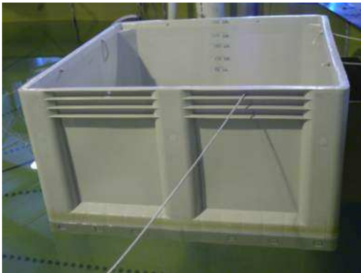
Volumetric Time-To-Fill Tank
