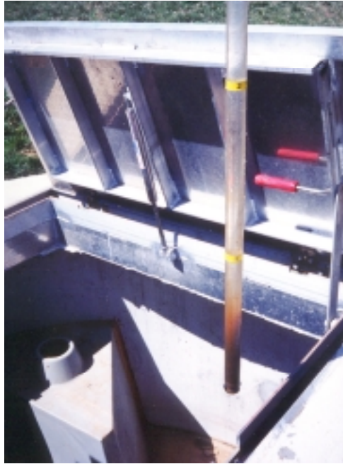
Figure 31. Isolater: Sediment Depth Measurement by Use of the Corer on 3/31/00
