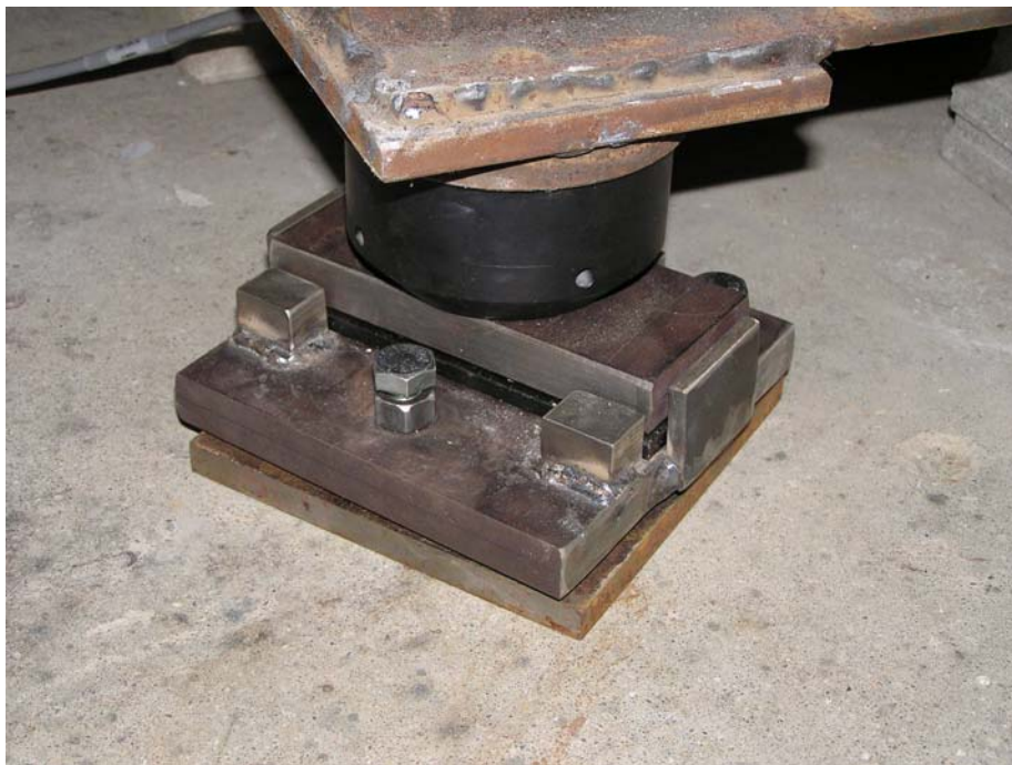
Figure 5 Load cell mounted on a transfer plate
