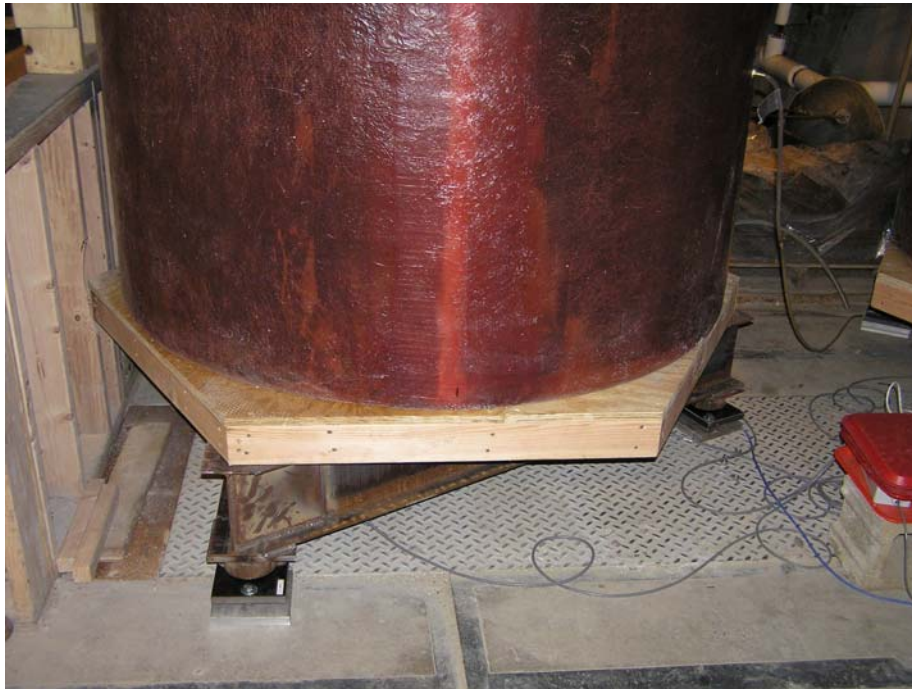
Figure 4 Support system of the M2 manhole
