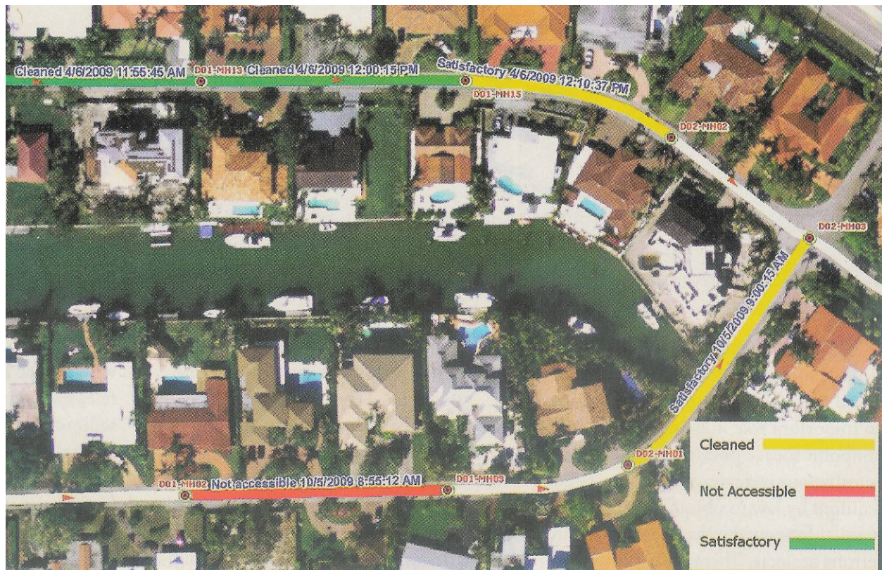
Figure 3-C.4. Commercial GIS Application Showing Storm Sewer Maintenance
