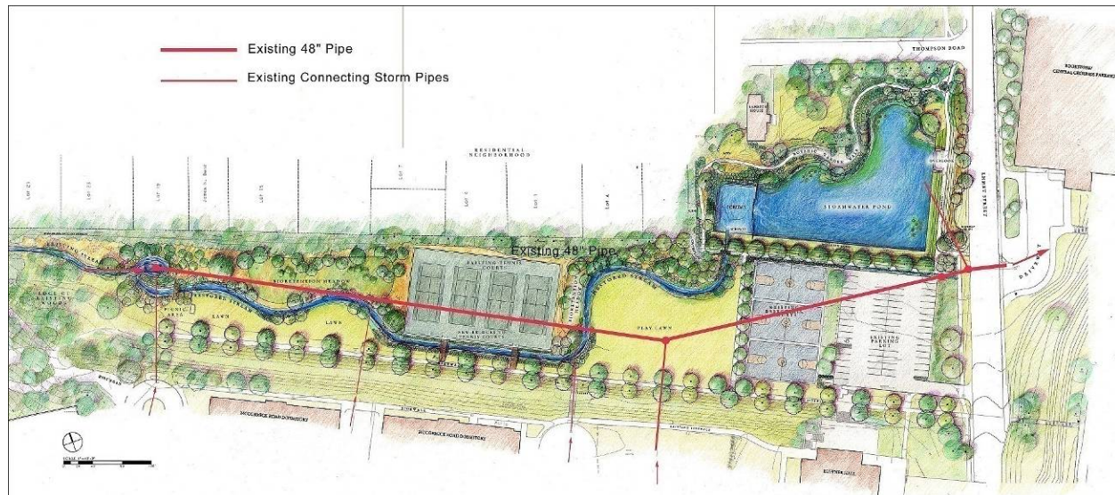
Figure 6.106. The UVA Dell Project Site. Location of the Piped Stream, Connecting Pipes, and the Daylighted Stream Configuration. Source: Nelson Byrd Woltz Landscape Architects
