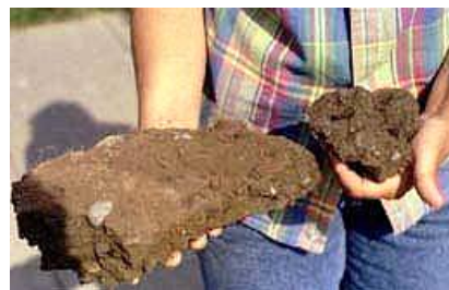
Figure 6.22. Compacted Soil Source: Center for Watershed Protection
