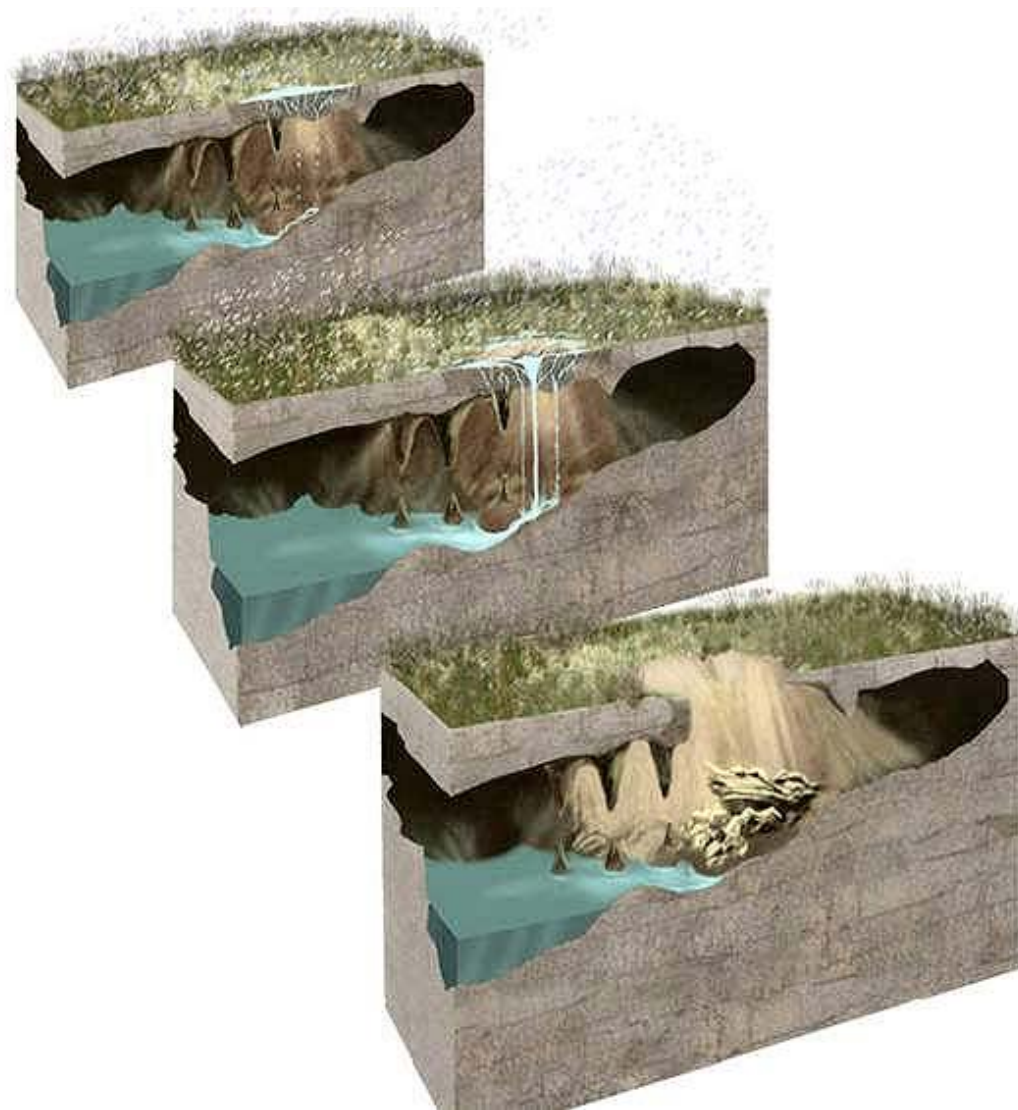
Figure 6-B.5. Schematic of Sinkhole Formation
