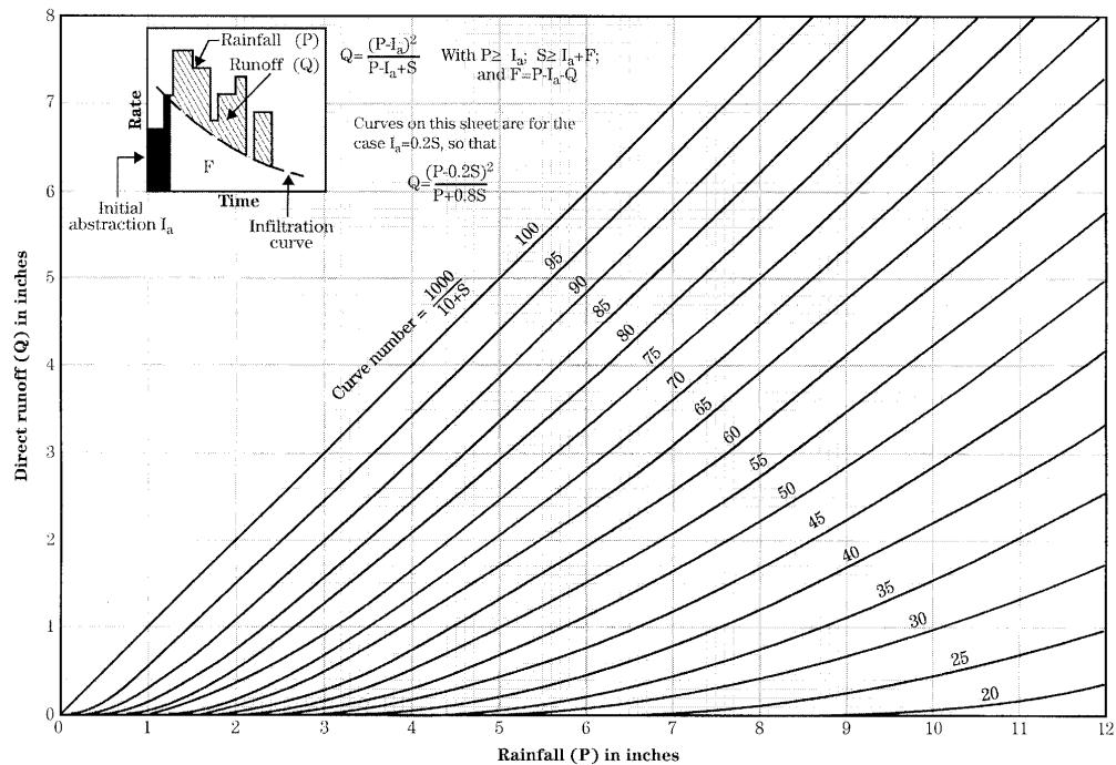
**Figure 11-C.1. NRCS Graphical Solution to Determine Runoff Depth from Rainfall Depth**
