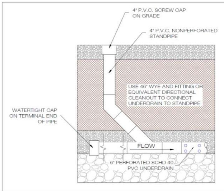
Figure 9-B.1. 4" P.V.C. Cleanout Detail
