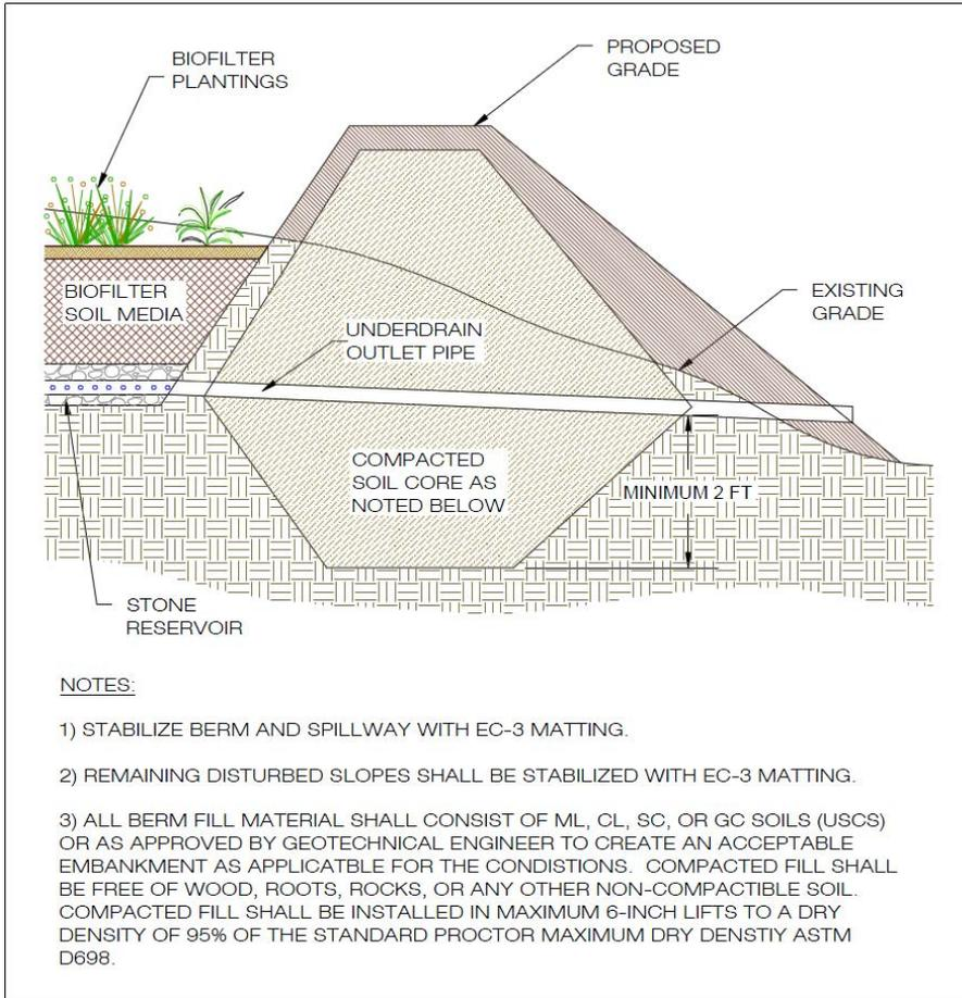
**Figure 9-B.2. Typical Bioretention Basin Berm**
