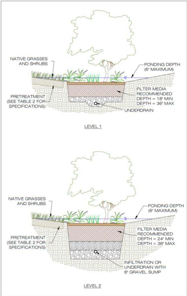
Figure 9.3. Typical Micro-Bioretentation Basin (Rain Garden) Level 1 and Level 2
