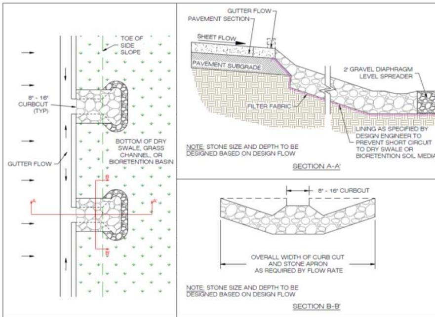
Figure 9.9: Pre-Treatment – Gravel Flow Spreader for Concentrated Flow
