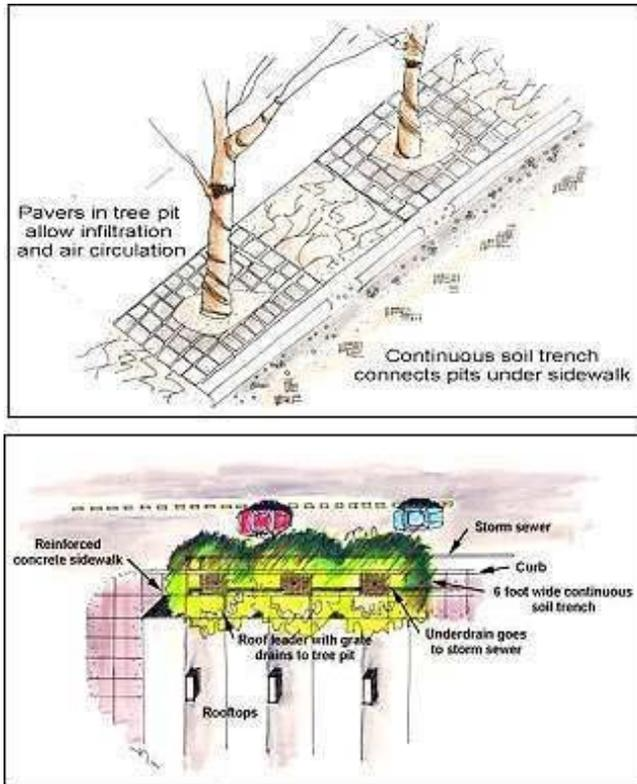
Figure 9-A.5. Expanded Tree Pit Details
