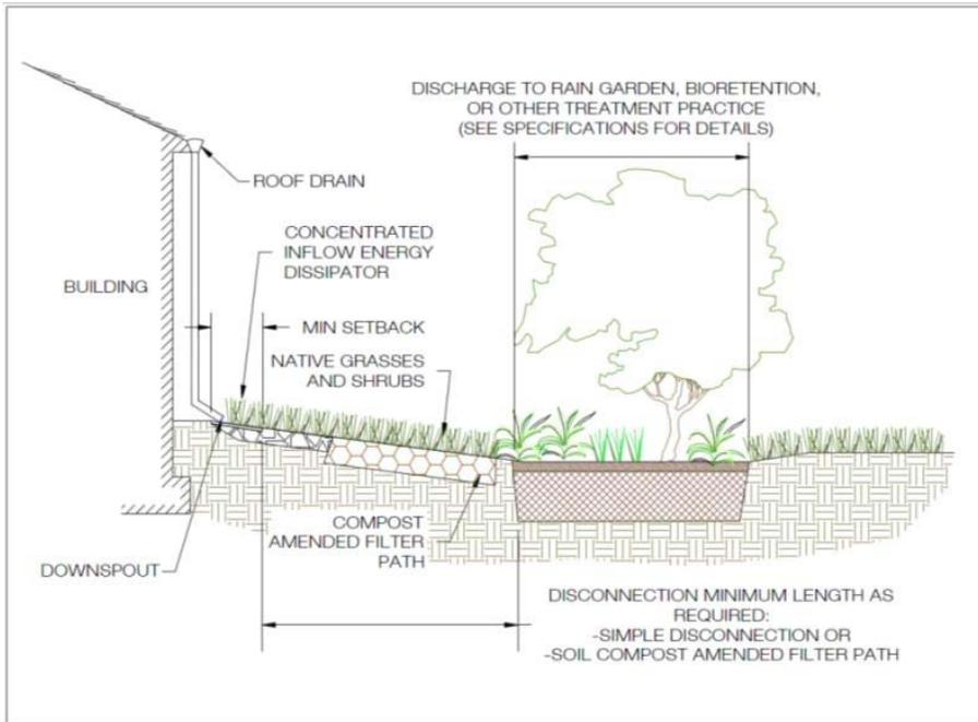
**Figure 9.2. Rain Garden (Micro Bioretention):**
