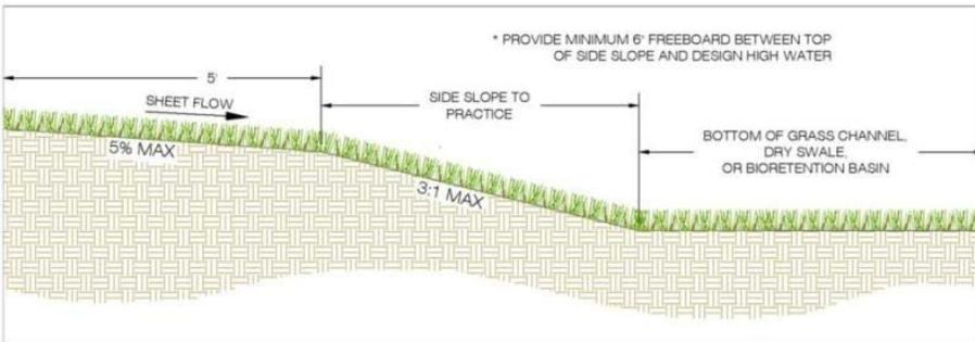
Figure 9.7b. Pretreatment II – Grass Filter for Sheet Flow
