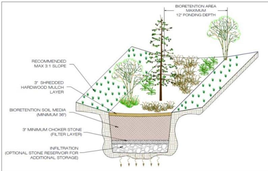
Figure 9.4b: Typical Bioretention Basin Level 2: Infiltration
