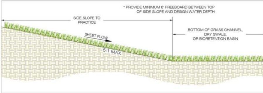
Figure 9.7a. Pretreatment I – Grass Filter for Sheet Flow
