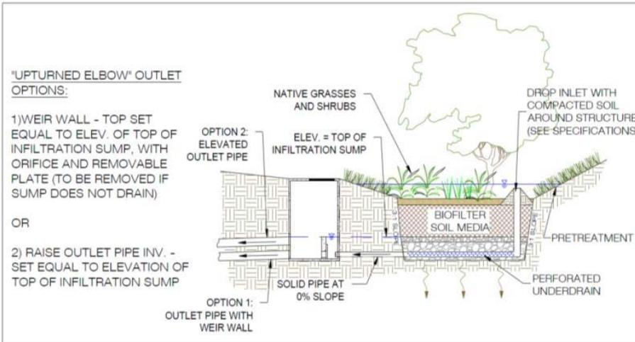
Figure 9.4d: Typical Bioretention Level 2: Infiltration Sump with "Upturned Elbow" or Weir
