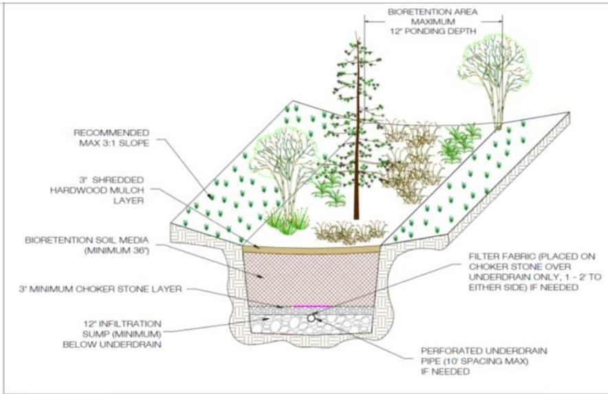
Figure 9.4c: Typical Bioretention Basin Level 2: Infiltration Sump
