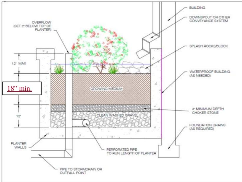
Figure 9-A.4. Stormwater Planter Cross-Section
