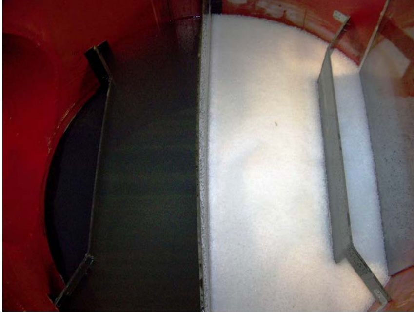
Figure 17 SciClone™ Inlet Loaded with LDPE Beads
